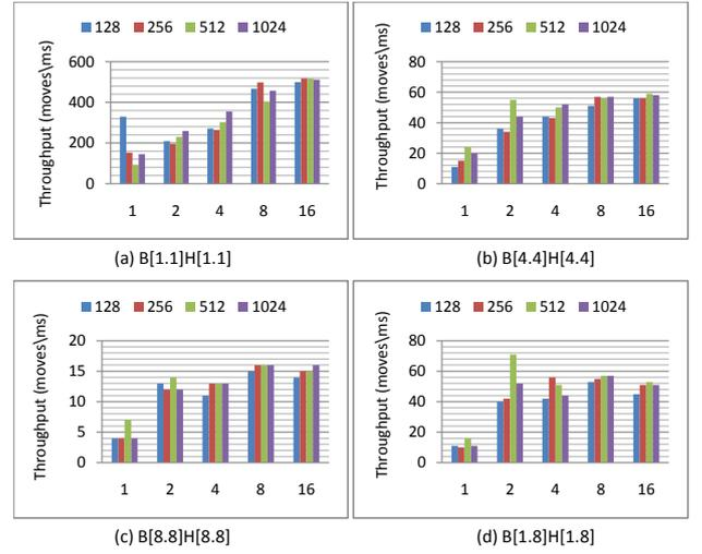
**Figure 4:** Relationship between throughput (total number moves per millisecond), BenchWorld size and the worm's body length and head size (higher values are better). (a) all worms have body length and head size 1; (b) all worms have body length and head size 4; (c) all worms have body length and head size 8; (d) both the body length and head size of every worm is randomly selected from the range [1, 8].
