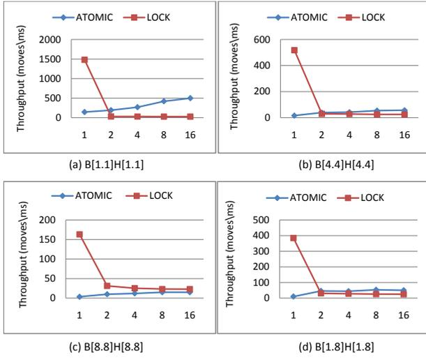
**Figure 3:** Comparing the performance between lock based synchronization and transactional memory synchronization (higher values are better). (a) all worms have body length and head size 1; (b) all worms have body length and head size 4; (c) all worms have body length and head size 8; (d) both the body length and head size of every worm is randomly selected from the range [1, 8].
