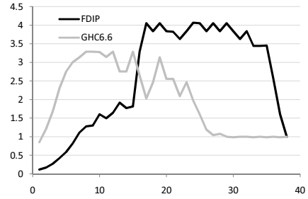
Figure 10. Parallel speed-up on a 4-core processor (y-axis) against thunk granularity (x-axis) for GHC 6.6 and for the modifications we introduced to support FDIP. For this workload the GHC 6.6 implementation provides a better parallel speed-up for very short-running thunks, but the FDIP mechanisms provide a near-optimal 4-fold speed-up for the longer thunks that we are interested in.
